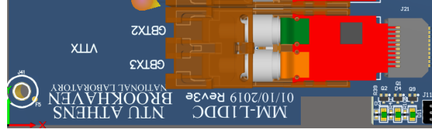
Figure 4.11: Cutout implemented in production boards for the cooling of the VTTX and VTRX.
