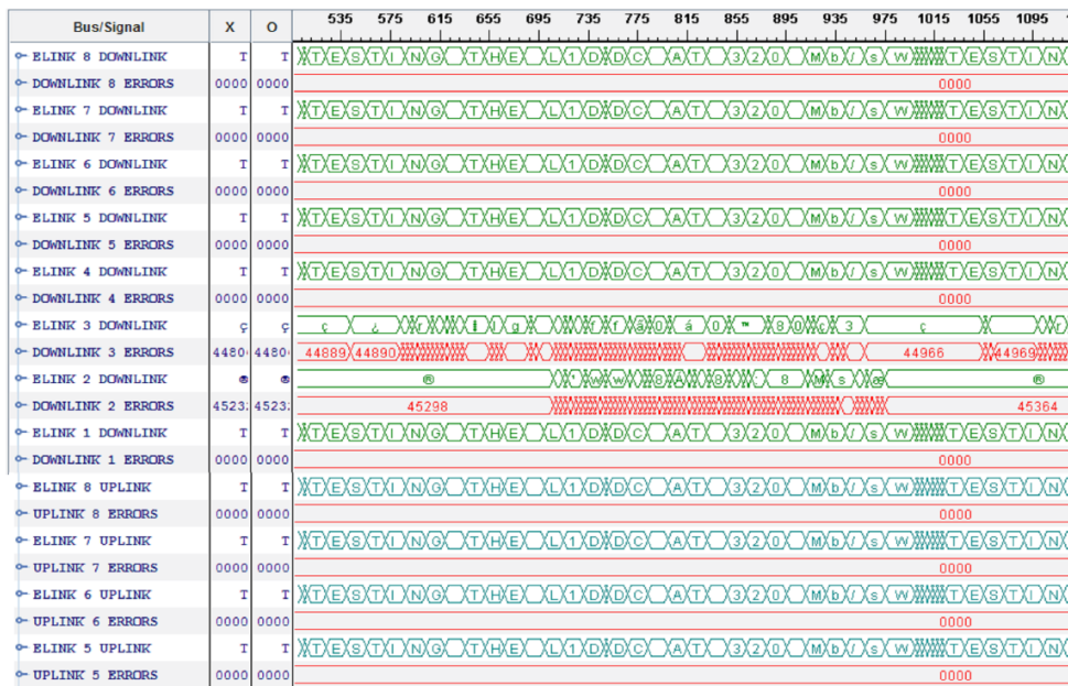
Figure 2.10: E-Link testing of the L1DDC prototype-1 board.
