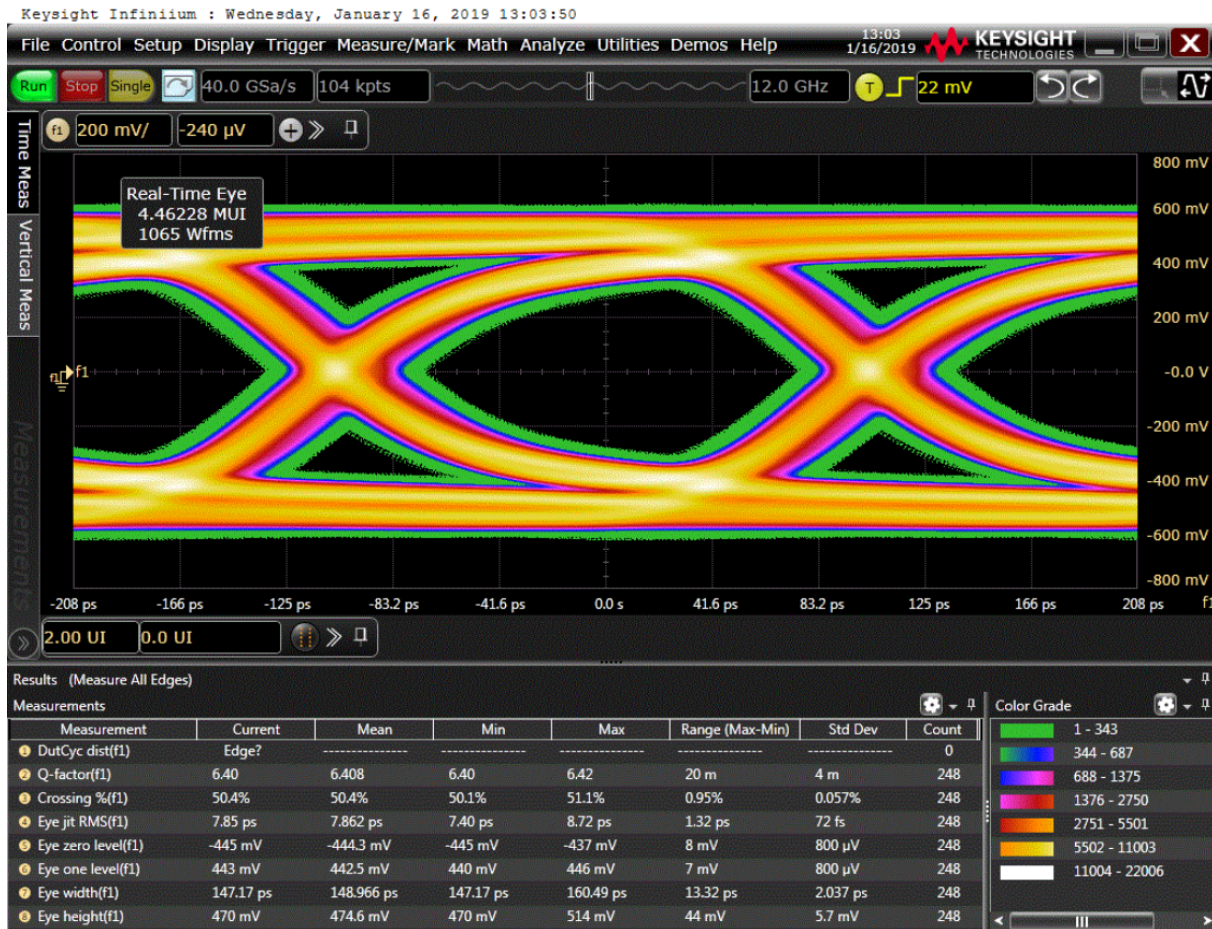
Figure 6.10: Eye diagram for 4.8 Gb/s data from sFEB with 8 m twinax cable and repeaters.
