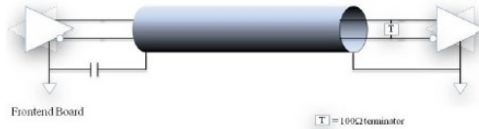
Figure 1.25: Grounding policy for the NSW electronics.
