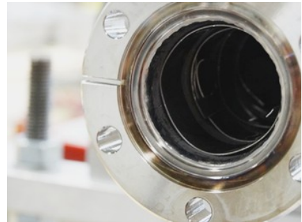
Figure 3.3: Witness samples placed inside the test pipes at their entrance before the start of the experiments
