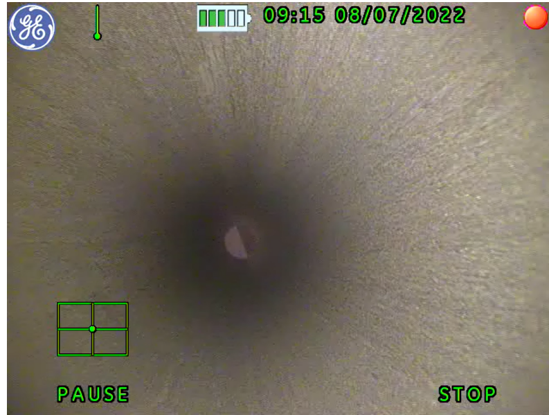
Figure 4.29: Perspective view of the TiZrV coating during the endoscopy after the low pressure experiment
