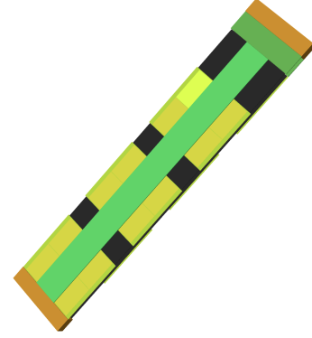
(b) Stave with three ATLASPix3 modules on both sides
