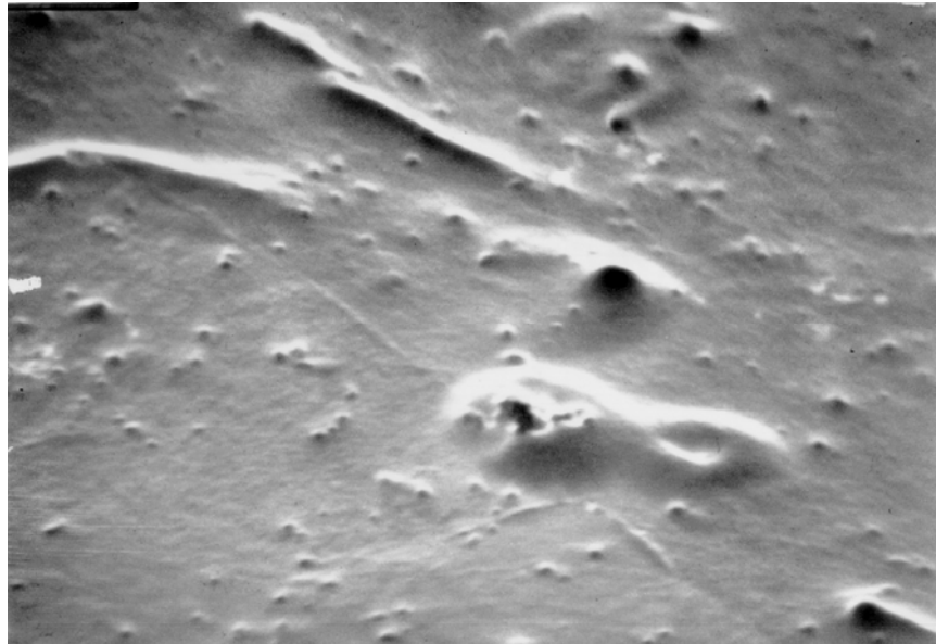
Figure 3. SEM photograph showing the surface morphology of a copper sample after chemical polishing of 80 \mu\text{m} .
