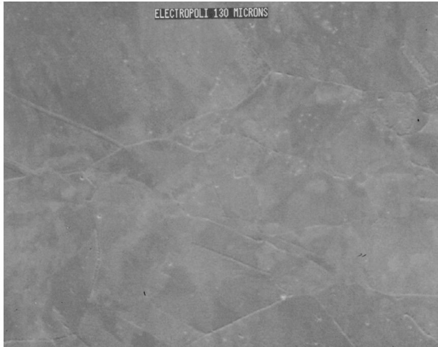
Figure 7. SEM photograph showing the surface morphology of a copper sample after electrochemical polishing of 130 \mu m ( \times 2500 ).
