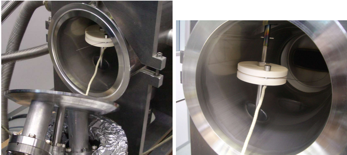
Figure A.3: These pictures show the opened front aperture of the pre-chamber. The rotatable device for stretching the wire can be seen, as well as the insulated transition from the wire to the RF-input, integrated in the front flange.
