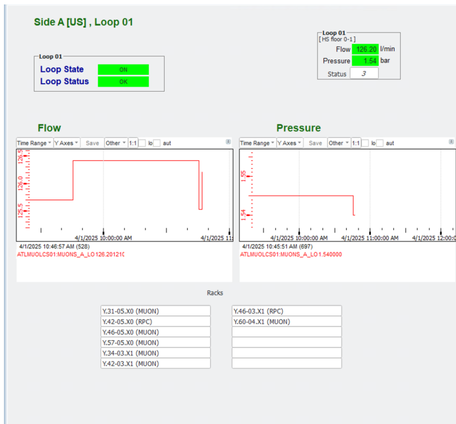
Figure 3.20: The Main FSM Panel that gives information for every loop
