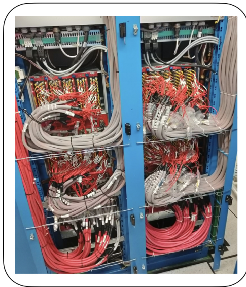
Figure 3.27: The HV units and racks at different stages of HV connections are shown.
