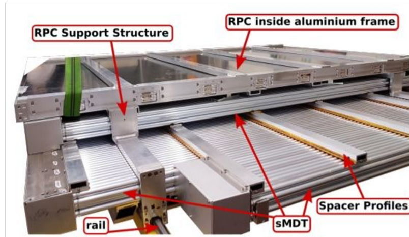
Figure 2.10: The BIS78A chambers as they are positioned into the ATLAS MS
