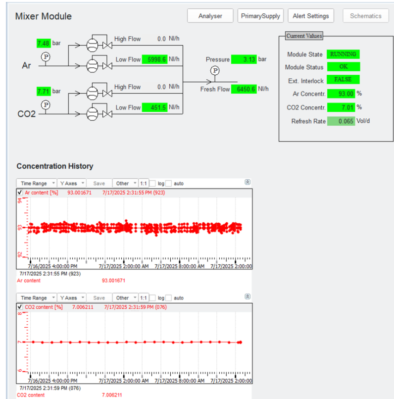
Figure 3.69: The main FSM panel Gas Panel for the Gas Mixer
