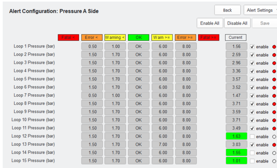
Figure 3.18: The Alarm limits of Muon Cooling
