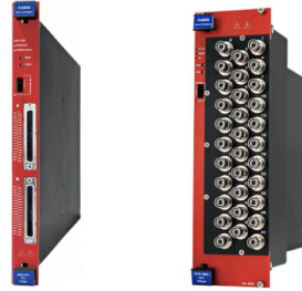
Figure 3.24: CAEN’s A7038AP (left) and A7038ST(N/P) (right) boards used in the high voltage connections for MM are shown.
