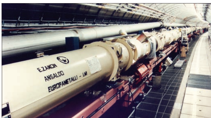
A view inside the 6.3 km tunnel of HERA shows the superconducting magnets – used to guide the proton beam – installed above the normally conducting magnets of the electron ring. (Courtesy DESY.)
