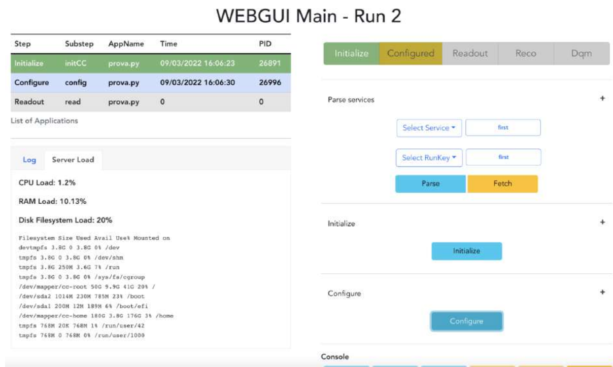
Figure 6.22: The main MTD web-GUI page for data acquisition. At the top of the left column, the GUI displays the executed commands (green), the running command (cyan) and the upcoming commands (grey). In the bottom left, the GUI displays live information from the Serenity backend about CPU, RAM and disk loads. At the top of the right column, the GUI displays the status of the backend FSM and the panels for the selection of the configuration files and for triggering the actions.
