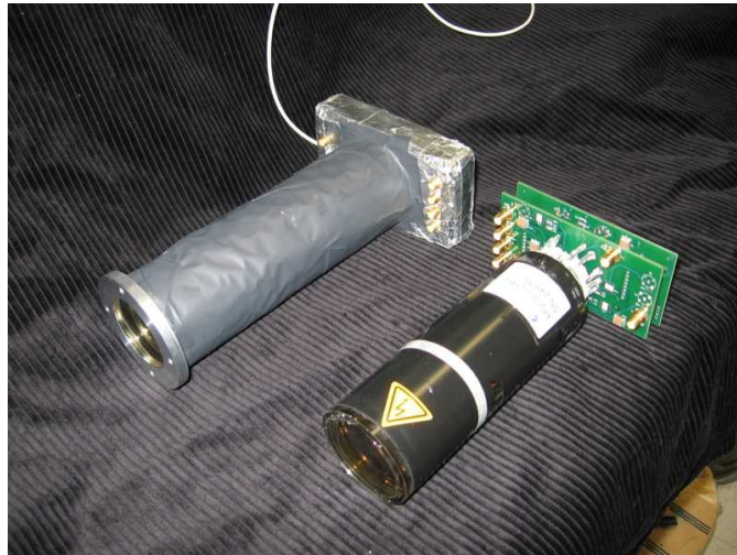
Fig. 3.3 Two CREAM TCD XP2020 PMTs being prepared for installation. The tube on the right has been mounted to the PMT active base circuit boards (Chapter 4). The tube on the left has also been potted and grounded to prevent HV breakdown, had a Lucite extender and aluminum mounting ring attached (for coupling to the light guide) and wrapped for light-tightness. Not visible here under the light-tightening are two layers of \mu -metal for shielding from the magnetic field of the earth.
