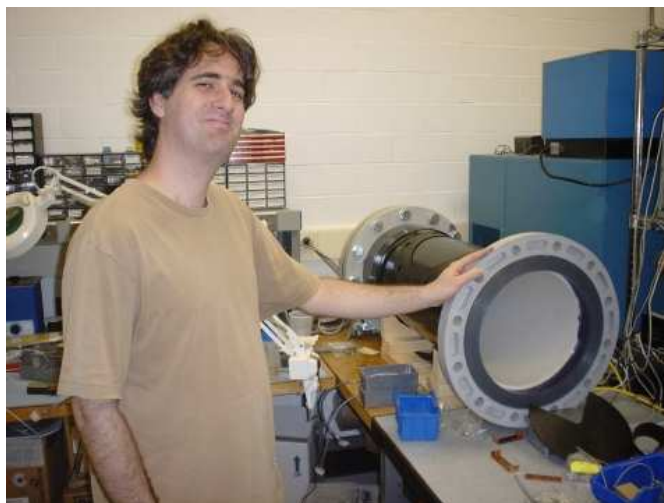
Fig. 3.11 PVC vacuum chamber for PMT/HV testing at Penn State. The chamber consists of a center section of PVC sewer pipe, with end-caps. The center section has been light-tightened with a layer of Tedlar and electrical tape. One end-cap contains piping for the vacuum pump and venting, the other contains BNC electrical feed-throughs (neither end-cap shown).
