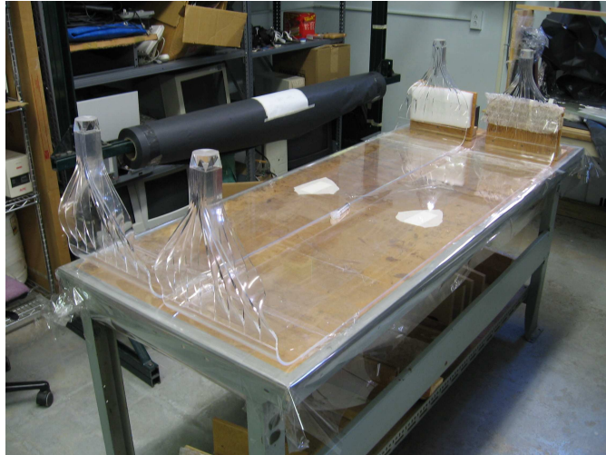
Fig. 3.2 Two CREAM TCD scintillation paddles after gluing but before wrapping for light tightness.
