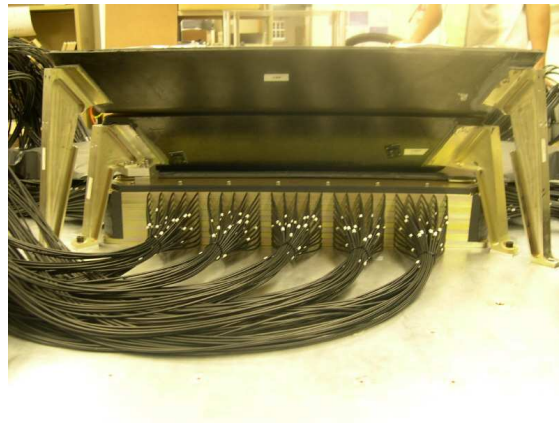
Fig. 2.4 CREAM II calorimeter stack during integration. The bottom structure is the calorimeter with fiber-optic readout visible. Above the CAL are the two carbon targets, with supporting metal pedestals at the corners.
