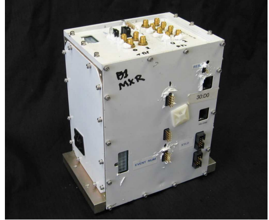
Fig. 3.10 CREAM electronics box refurbished and fully assembled. Visible on the top are gold-plated SMA headers from anode and dynode PMT signals. Each box takes input from two adjacent PMTs in the TCD. Also present on the top and side are connections for Ethernet, serial, trigger, event number input, and power input.
