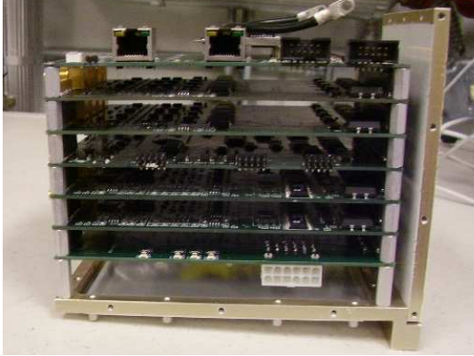
Fig. 3.9 CREAM TCD electronics box (Concentrator). The boards (from bottom to top) are: power board, two peak detector ADC boards, a local trigger board, two TDC boards and the on-board computer board. The computer [12] actually resides in a small daughter-board at the very top of the stack.
