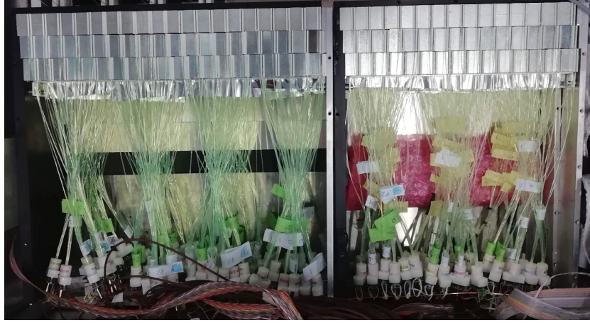
Figure 7.2: Lateral scintillation light readout prototype
