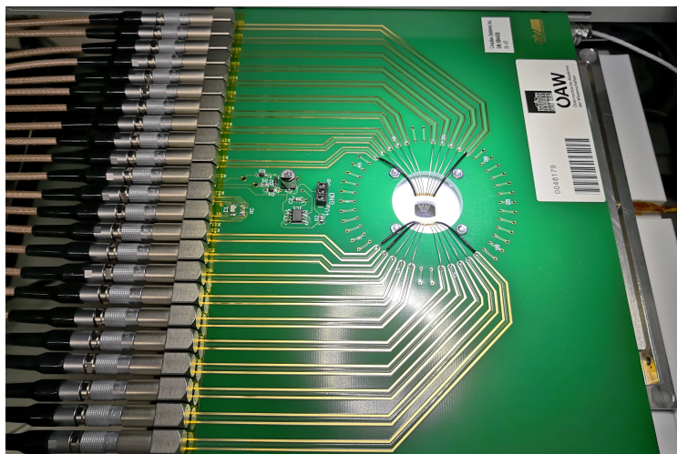
(A) Top view photograph of the PQC probe card with triax cables and LEMO connectors.
