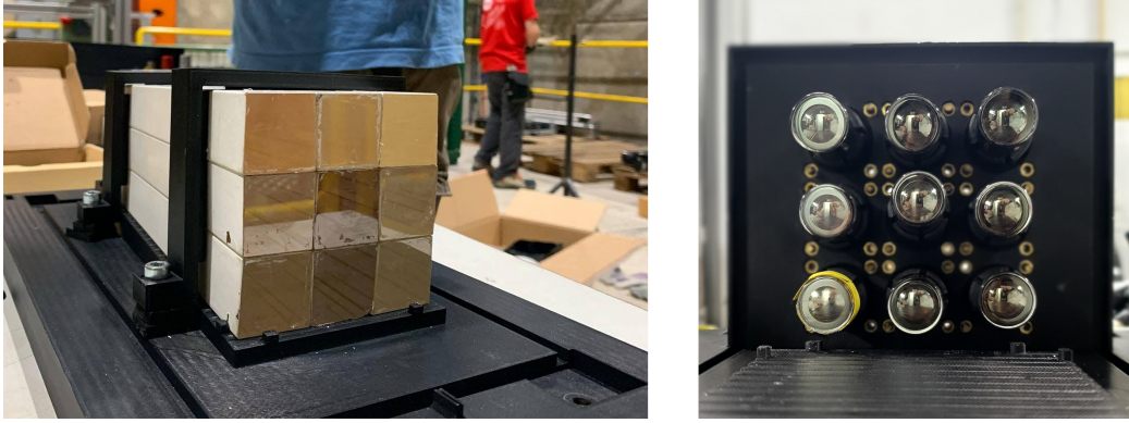
FIGURE 2.13: The Genni calorimeter: pictures of ( left ) the crystal matrix and ( right ) the PMT matrix.
