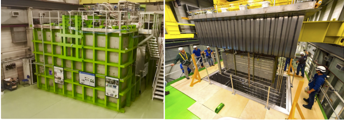
Figure 3.17: Pictures of WA105 3 \times 1 \times 1 \text{ m}^3 Dual-Phase LAr-TPC demonstrator. Left: Outer view of the cryostat. Right: the TPC is suspended under the top cap during its insertion in the cryostat [143].
