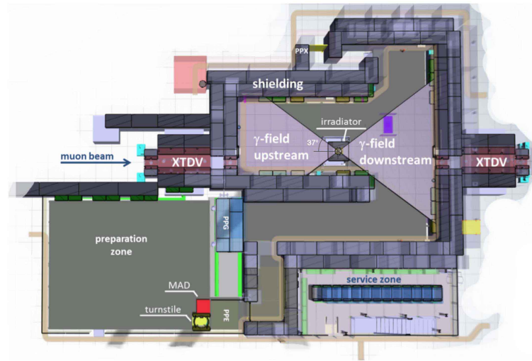
Figure 2.1: Inside view of GIF++ irradiation bunker with the indication of two different regions: upstream and downstream.
