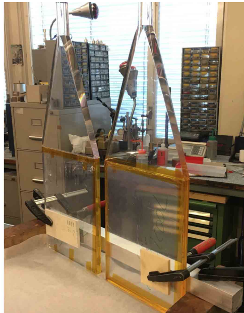
Figure 2.15: On the left, technical drawing of the detector used for the beam trigger system. The distances are in millimeter. A photo of the assembly of scintillators (on the bottom) and light guide (on the top) is present on the right. The optical cement resin (EJ-500) and hardener are used in the interface.
