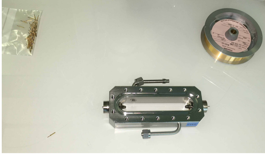
Figure B.1: Picture of a SWPC built for the experimental setup at GIF++. In the photo, you can see the main structure of the SWPC, the gold-plated tungsten wire and the pins, which will be fixed to the wire by clamping.
