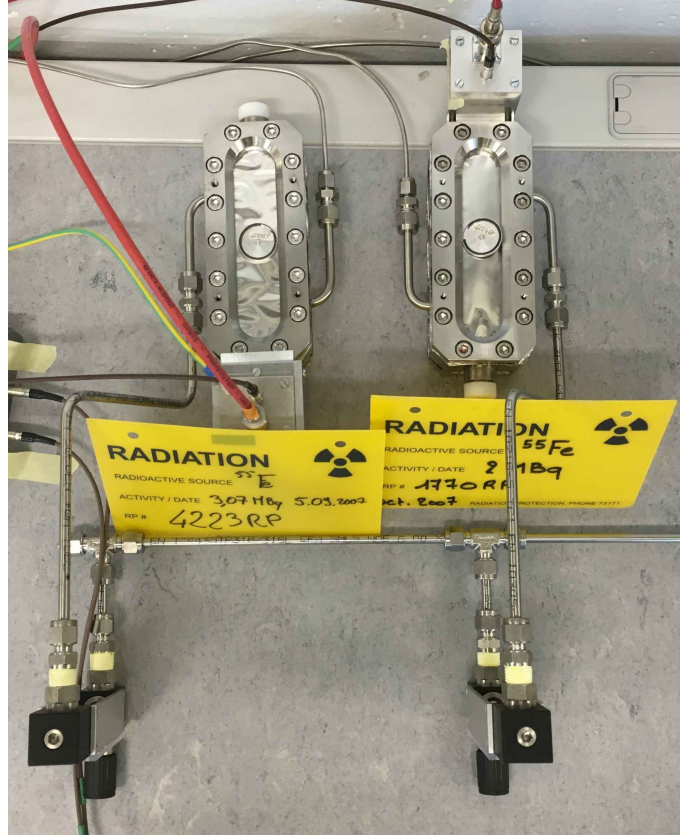
Figure B.5: Experimental set-up for the characterization of the SWPCs in the laboratory. In this picture, the radioactive source of ^{55}\text{Fe} are placed in the middle of aluminium window (position 3). For convention, the position 1 is close to the HV module. The experimental conditions are specified in chapter 3.
