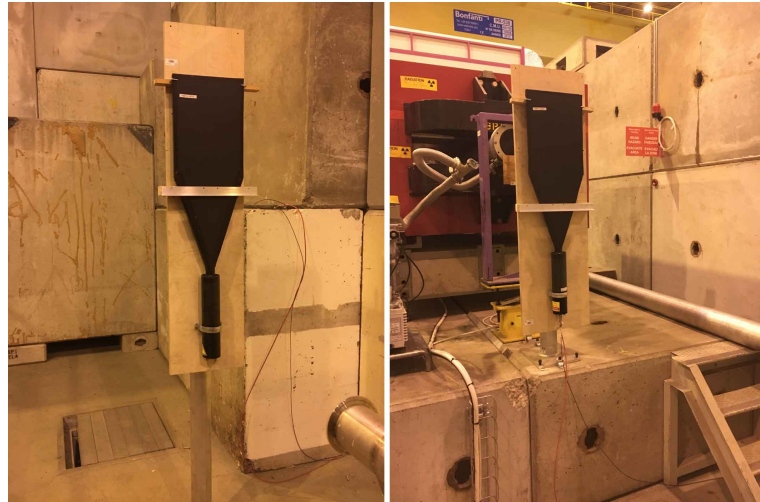
Figure 2.25: On the left there is the photo of detector 1, placed in the upstream region outside the bunker; whereas the detector 2 (on the right in the figure) is located in downstream region between GIF++ and the facility CMS-ECAL.
