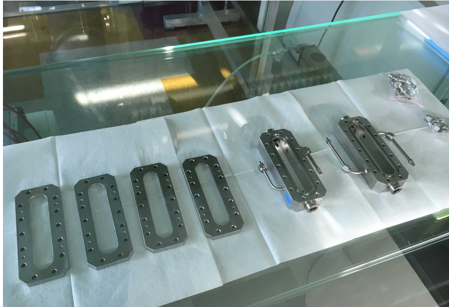
Figure B.2: Components of the SWPCs in the clean room.
