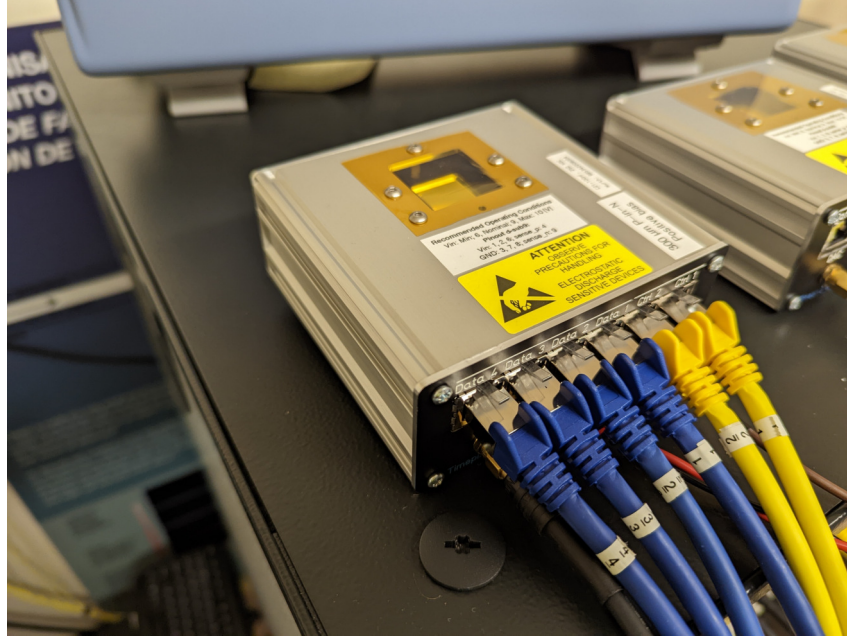
FIGURE 10: TIMEPIX3 BEAM LOSS MONITOR (BLM) ASSEMBLY. THE CHIP IS LOCATED BELOW ORANGE FOIL, WHICH IS PREVENTING DUST FROM ENTERING THE DEVICE. CONTACTS FOR THE POWER, BIAS VOLTAGE AND DIGITAL TO ANALOG CONVERTER (DAC) READING ARE LOCATED BELOW THE ETHERNET CABLES FOR CONTROL AND DATA CHANNELS.
