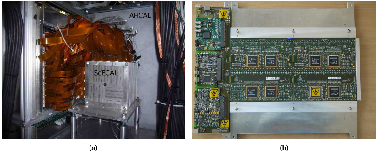
Figure 4.2 – a) Photo of the ScECAL physics prototype with the Fe-AHCAL at FNAL. b) Photo of the top side of a layer of the technological ScECAL prototype.
