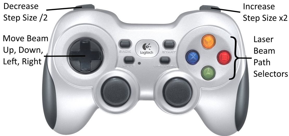
Figure 30: Wireless gamepad to control the picomotor Piezo Linear Actuators of the RILIS launch mirror optomechanics.
