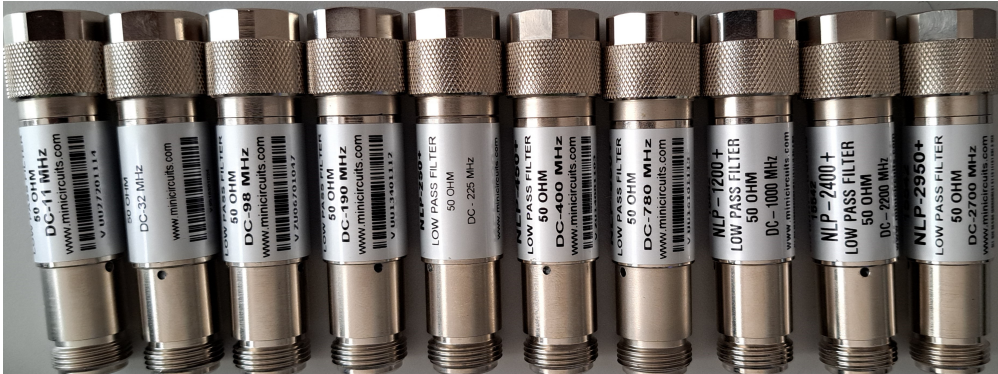
Figure 3: The ten low-pass filters that are used for ENOB measurements. They are from the NLP series from Mini Circuits.
