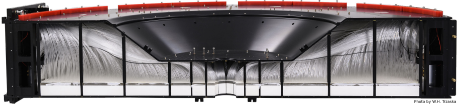
Figure 3.61.: Side view cross section of the FV0 detector [63]
