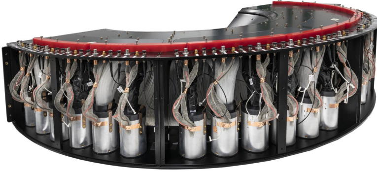
Figure 3.60.: Photograph of the semi-assembled FV0 focusing on the PMTs [63]
