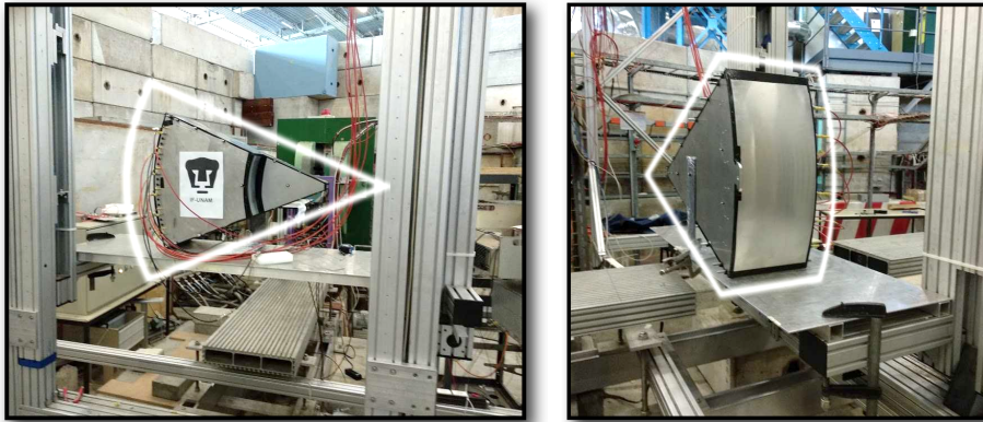
Figure 3.55.: Photographs of single-sector FV0 prototype installed at T10 beam-line at CERN's East Hall. The prototype is highlighted with white envelope
