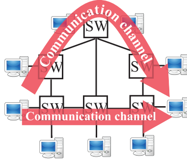
Figure 3.3: The path over an Ethernet network is considered an erasure communication channel.
