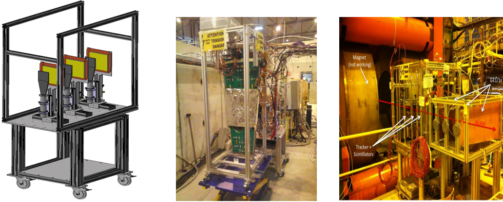
Figure 3.27: (left) Design of the tracking telescope showing three triggering scintillators (in grey colour), 10 cm \times 10 cm tracking GEMs (in yellow colour), (middle) a photograph of movable aluminum stand holding actual GE1/1 chamber in front of the tracking telescope during H4 beam test campaign, and (right) one of the earliest (December 2014) beam test setup at CERN SPS.
