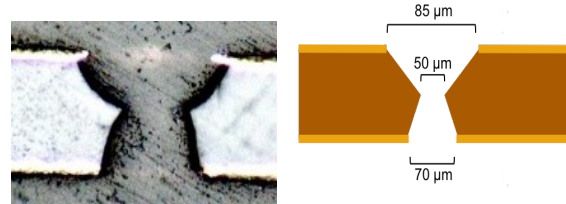
Figure 4.2: (left) Scanning Electron Microscope (SEM) image showing the asymmetric single hole structure in GEM produced by single-mask technique and (right) its schema.
