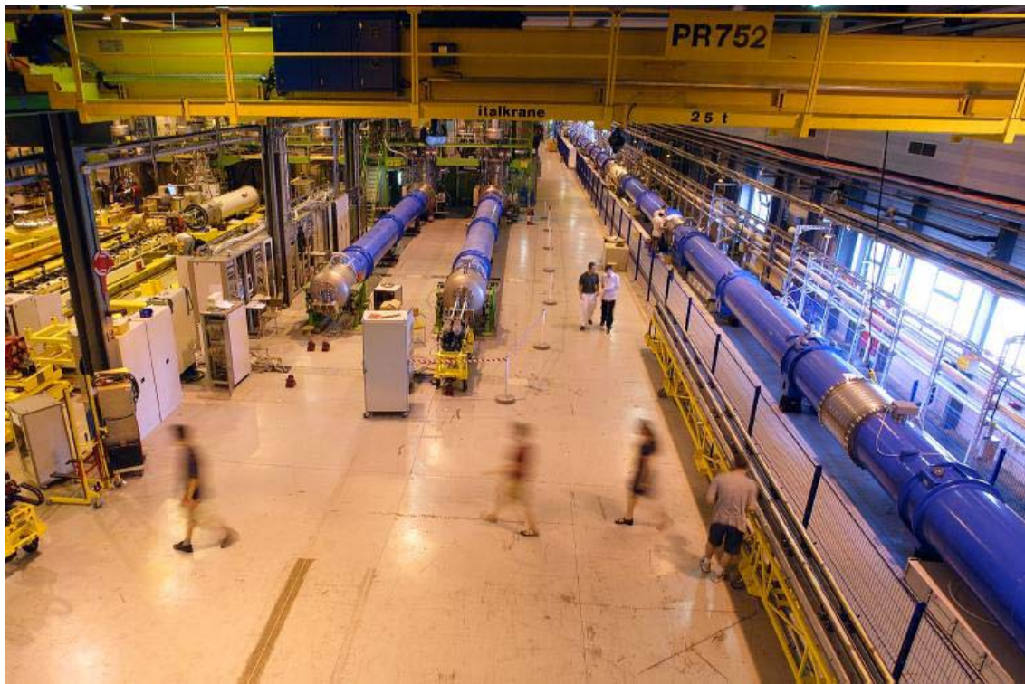
Figure 6.3: The LHC Test String-2 assembled in the SM18 building at CERN. The two individual magnet test benches can be also seen.
