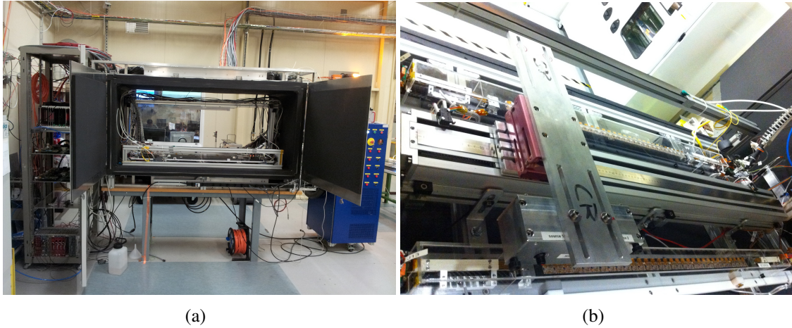
Figure 4.3: Stave QA test stand pictures showing the (a) outside and (b) inside of the environmental box.
