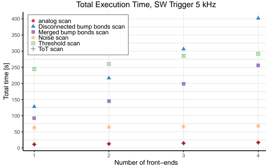
Figure 5.13.: The Total Execution time of analogue, disconnected bump bonds, merged bump bonds, threshold, ToT and noise scans as a function of the number of enabled FEs.
