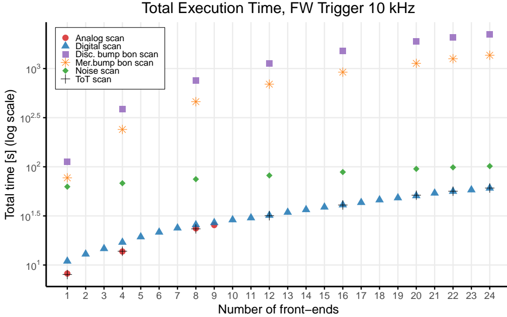
Figure 5.11.: The execution time of the scans as a function of the number of enabled FEs. Logarithmic scale.
