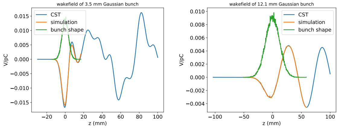
Figure 2.17: Wake potential for a BPM 3.5 and 12.1 mm Gaussian bunch obtained directly by CST (blue line) and with the convolution using the wake potential of 0.4 mm Gaussian bunch (orange line), the "pseudo Green-function".
