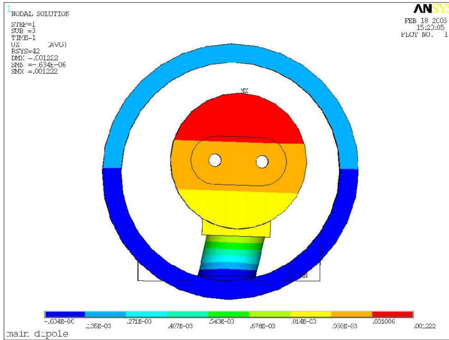
Figure 6.21: Effect of a 5 \text{ m/s}^2 lateral acceleration on a cryo-dipole equipped with ideal restraints. Lateral displacement [m] in the middle cross section.
