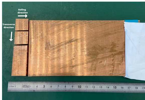
Figure 2: Representation of the cutting directions on Sample 2.
