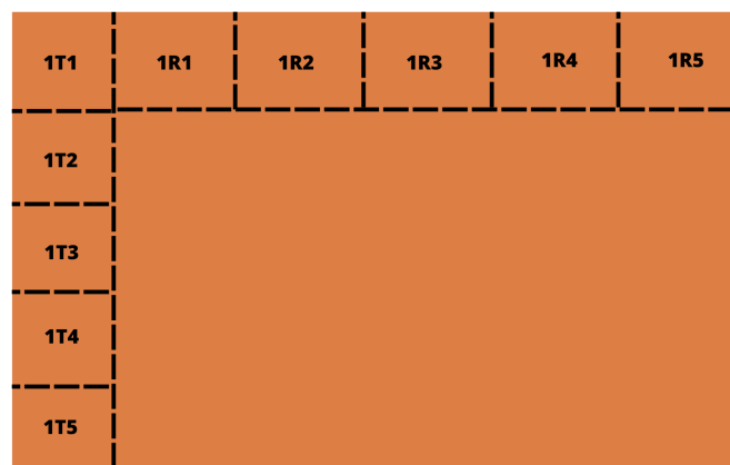
Figure 3: Representation of the cutted samples on the rolling and transverse direction for Sample 1.
