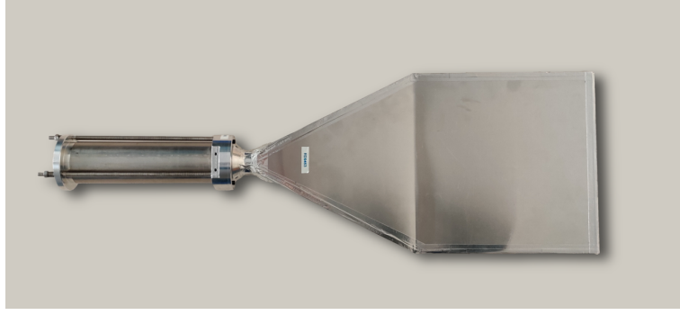
Figure 12.6: Photo of one of 30 cm \times 30 cm scintillator modules including the light guide.
