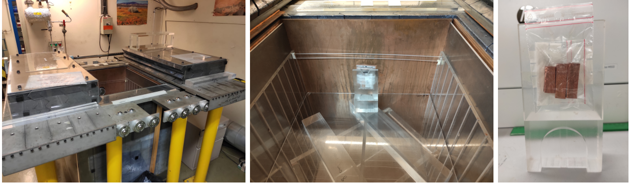
Figure 6.1: Pictures of the setup used in the gamma-ray spectrometry laboratory in building 24. GE5-B10162 detector open (left), interior of the detector with one of our radioactive samples placed and ready to be measured (centre) and detail of the samples and the support, used for an optimum alignment of the samples and the detector (right).
