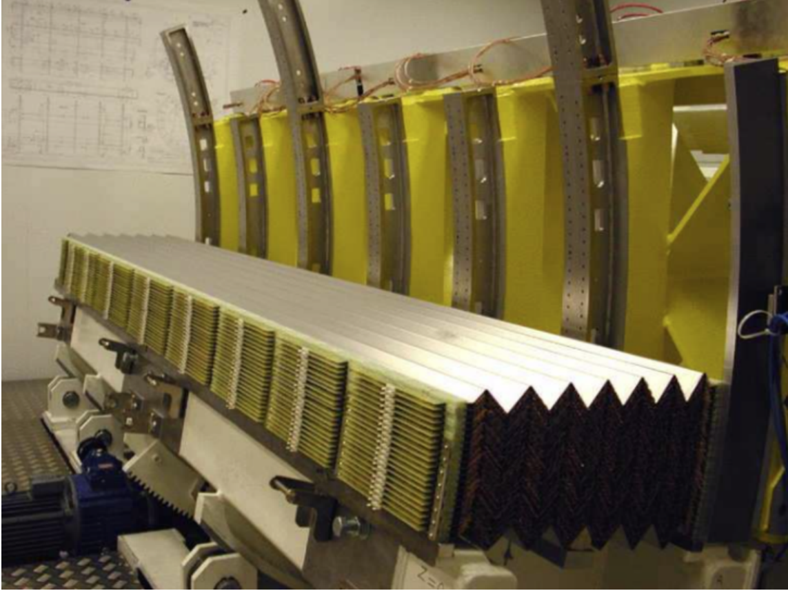
Figure 4.10: Photograph of a partly-stacked barrel EM LAr module [84]. Six out of seven outer support rings are also visible. The module and support rings rest on an assembly bench.
