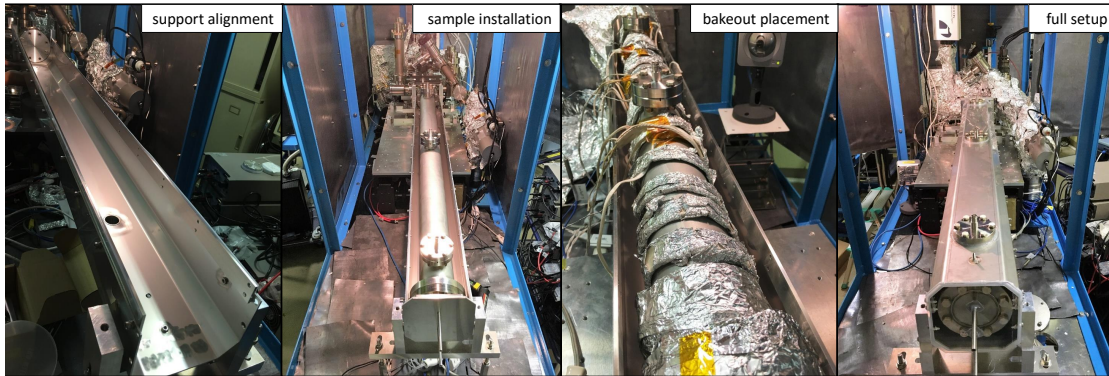
Figure 3.24: Assembly steps of the liquid N 2 cooled sample with the thermal insulating jacket
