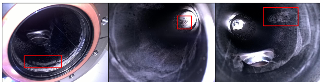
Figure 3.30: Amorphous carbon peel-off locations after the second coating attempt Photo: Antonios Sapountzis, CERN
