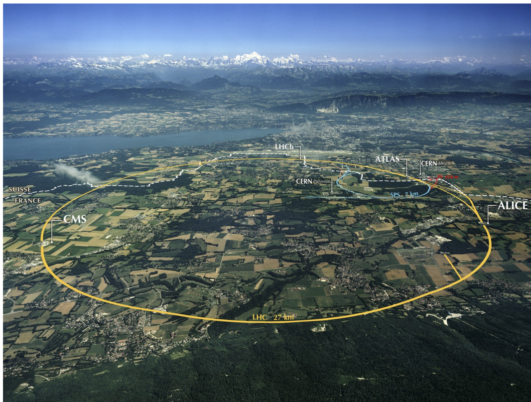
Figure 1.1: Aerial view of the LHC. The interim stages of the accelerator chain as well as the position of the four detectors is also shown [8].
