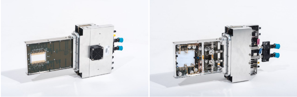
Figure 2.11: Sensor side (left) and cooling side (right) of an assembled GTK station. [103]
