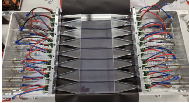
Figure 2.13: Bottom part of a VetoCounter station. [104]
