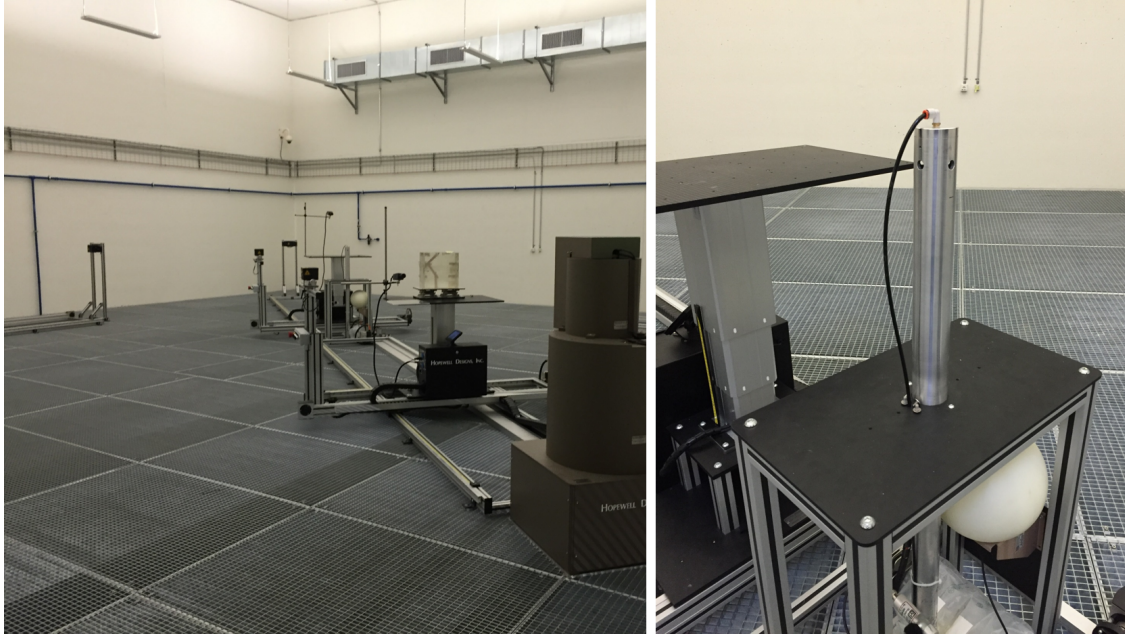
Figure 4.14: Am-Be irradiation room to the left and source exposure position to the right.
