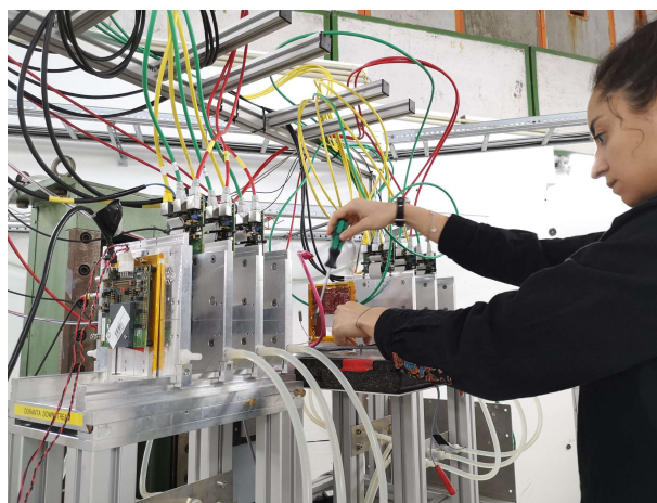
FIGURE 6.1: Mounting modules in DESY testbeam facility to be characterised with 5 GeV electron beam. Results in this chapter are produced from this setup.
