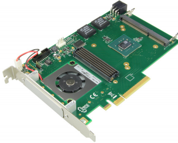
FIGURE 4.4: Image of a Trenz TEF1001 board, one of the PCIe FPGA FMC boards supported by the YARR firmware.
