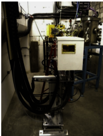
FIGURE C.2: The scanning system with the cooling box attached in the Birmingham irradiation facility [189].
