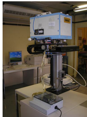
FIGURE C.3: Irradiation prototype table at the CERN PS Irrad facility equipped with thermostated irradiation box [190].
