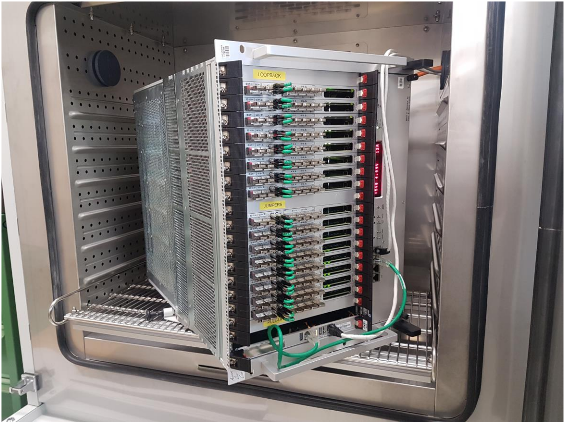
Figure 6.10: Fully setup VME crate inside the climatic chamber. The displayed configuration allows testing of 16 DUTs in parallel, all equipped with FMCs, LEMO connectors and SFP loopback modules.
