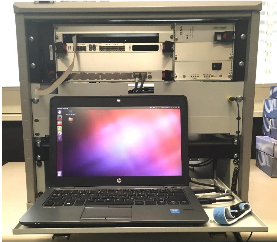
Figure 6.8: Test bench for the VFC-HD End-of-Line test. Each DUT had to be tested at once running the custom Production Test Suite.
