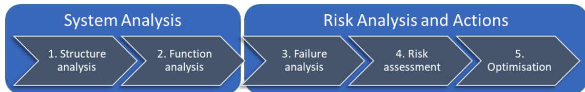
Figure 3.7: The five steps of the System FMEA, according to [78].
