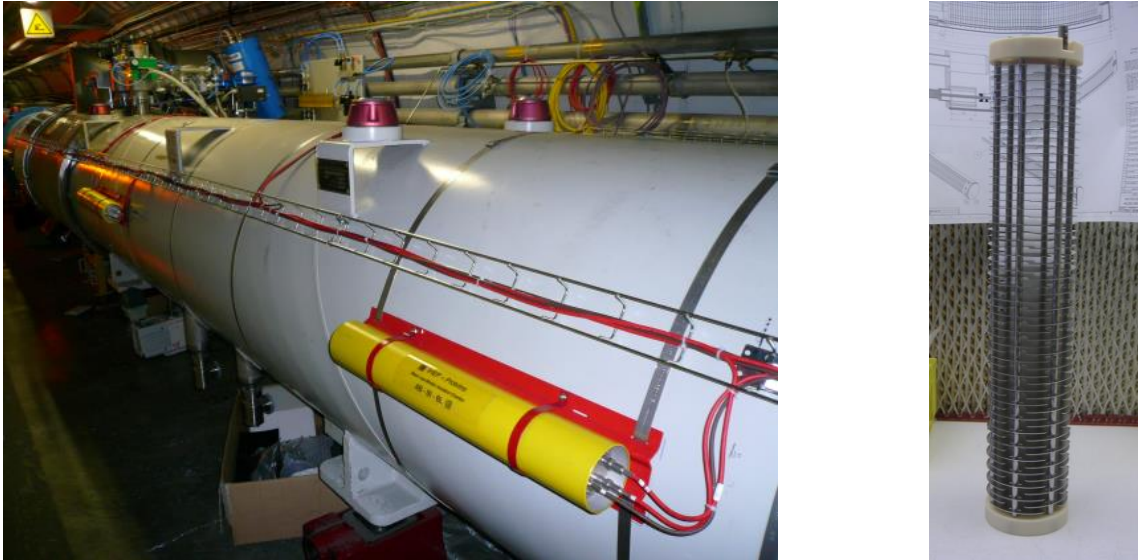
Figure 2.3: LHC BLM system Ionisation Chamber. Installed chamber on the LHC cryostat (left) and the inner multilayer capacitor with insulation (right).
