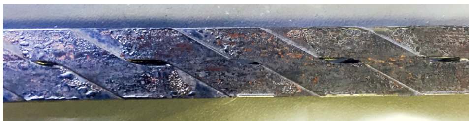
Figure 2.50. The Roebel cable after pre-soldering with the \text{Sn}_4\text{2Bi}_5\text{7Ag}_1 solder paste.
