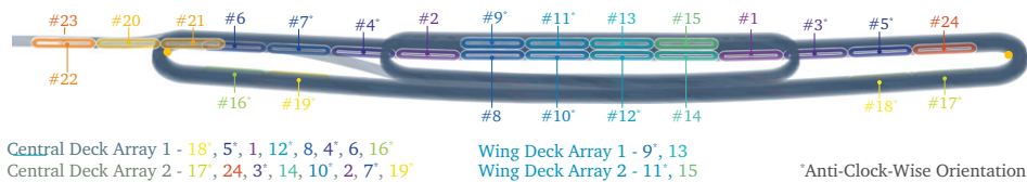
Figure 5.20. Possible position of pick-up coils when integrated inside Feather-M2. The asterisk denotes anti-clockwise orientation with respect to the outside of the magnet, otherwise the coil is clock-wise.
