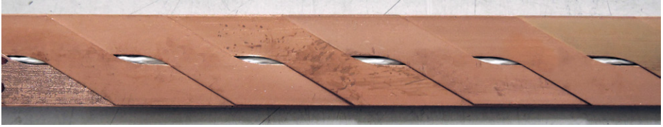
Figure 2.1. Photograph of a Roebel cable by KIT assembled from Bruker ReBCO tapes. The cable shown here was later used in the Feather-M0.4 coil. A glass fiber rope was inserted into the central channel (visible) before winding and impregnation.
