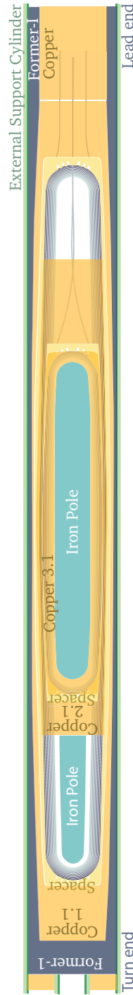
Figure 2.48. Illustration of the horizontal longitudinal cross-section of the Feather-M2 magnet at a height of 22 mm. Only the top former is visible, together with the coils, iron poles and copper rings that are mounted on it. In between the coil and the copper ring the overall shape of the spacers is visible. On the outside there is the external support cylinder.
