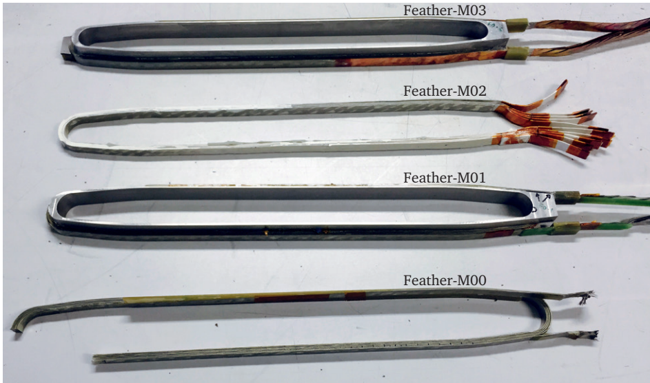
Figure 2.54. Photograph showing the series of Feather-M0 exercise coils side by side, produced to study the winding and impregnation procedures.
