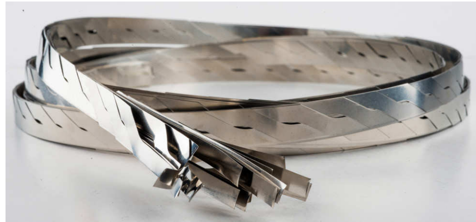
Figure 1.11. Photograph of a coiled Roebel cable (by Henry Barnard at CERN). This demonstrator cable was manufactured, using stainless steel tapes, at Karlsruhe Institute of Technology (KIT).
