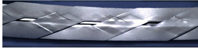
Figure 2.7. Photograph of a dummy Roebel cable made with stainless steel tapes after performing a bare 10-stack test up to 150 MPa overall pressure. The cable shown was located near the middle of the stack. It can be seen that the surface pattern of the adjacent cable is heavily imprinted in the tape.
