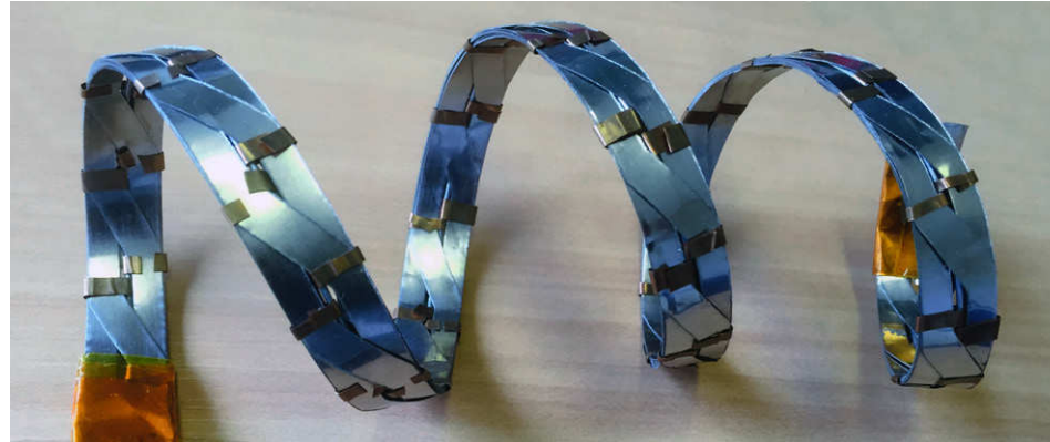
Figure 2.12. A three-turns spiral with about 40 mm diameter for demonstration of the bracelet method for mechanically stabilizing the Roebel cable.
