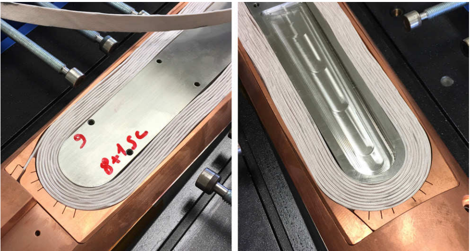
Figure 2.63. Photograph of the lead-end (left) and the turn-end (right) of Feather-M2.0 after winding of the central deck and the mounting of the copper rings (step III in Figure 2.62). Visible are the individual turns, the copper spacer and ring, the former and part of the winding and impregnation tooling.
