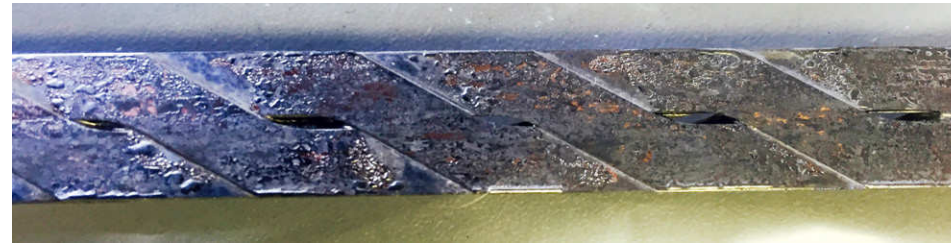
Figure 2.50. The Roebel cable after pre-soldering with the \text{Sn}_{42}\text{Bi}_{57}\text{Ag}_1 solder paste.
