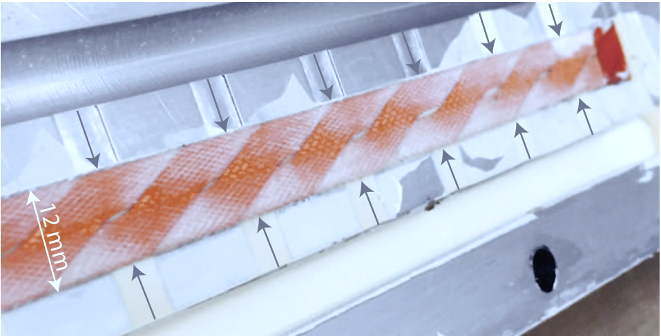
Figure 4.11. The impregnated sample in the specifically designed 300 mm long impregnation mold for single tapes at CERN. Visible are the channels that allow the resin to penetrate the cable from its edges.
