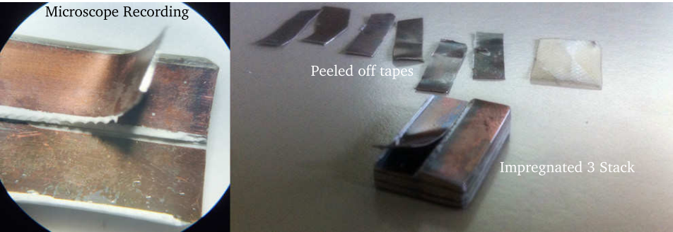
Figure 2.10. Internal inspection of an impregnated 3 stack of dummy Roebel cables. The tapes can be peeled off one by one because the resin did not enter in between the tapes.
