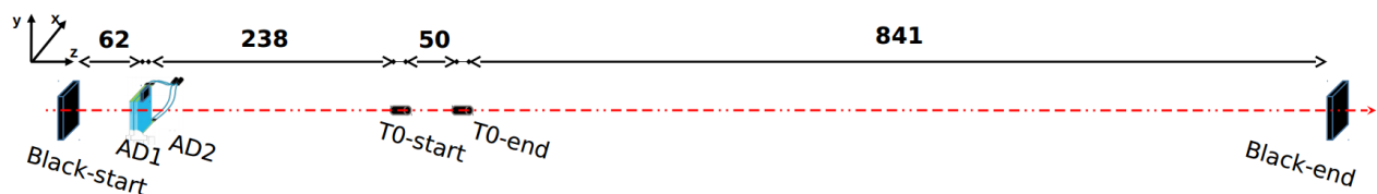
FIGURE 3.12. Beam test setup scheme at T10 beam line. Distances are marked in centimeters, and the red arrow show the direction of the beam.
