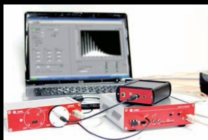
Set-up for SiPM testing & characterization
