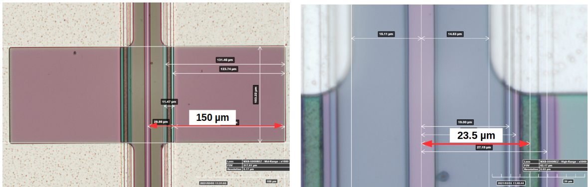
Figure 6.34. – Microscope images with different magnification of the interpad region of an HPK2 5x5 LGAD. JTE and p-stop structures can be identified.
