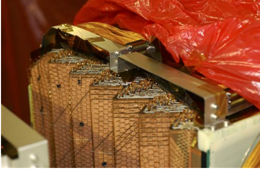
Figure 2.7: Characteristic accordion structure in EM calorimeter [64].
