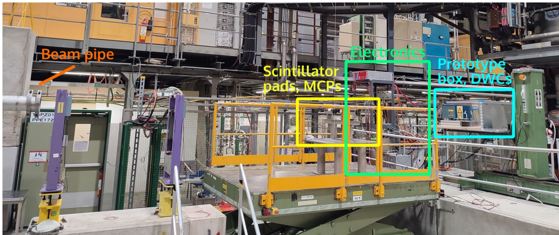
Figure 4.2: The test beam setup in June 2023 at SPS.
