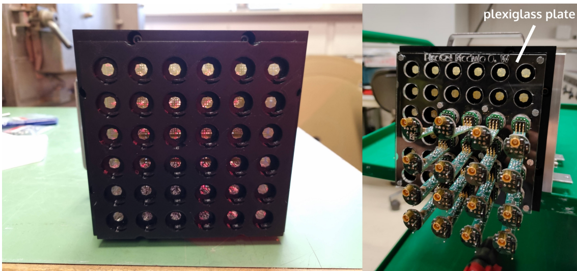
Figure 3.11: (a) "Clicking mechanism" of the hollow light guide. (b) An additional plexiglass plate mounted on the back side of the prototype with a set of screws.
