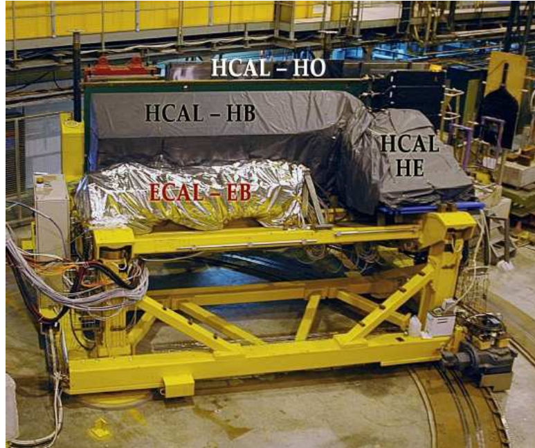
Figure 3.13: Photograph showing the platform used in combined HCAL/ECAL test beams.
