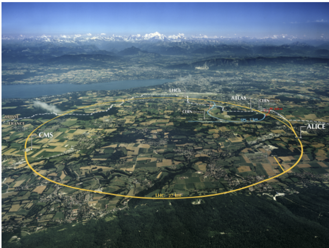
Figure 3.1: A schematic of the LHC ring and associated experiments overlaid on a photo of the surrounding countryside.
