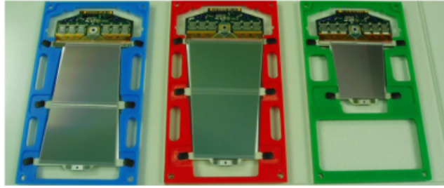
Figure 2.13: SCT endcap module types (outer, middle and inner).
