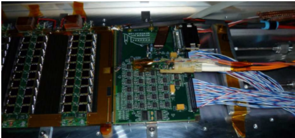
Figure 5.33: Position of the VersatileLink on top of the EoS card for one of the tests.
