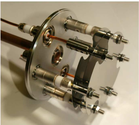
(b) Inside view of a SEM detector.
