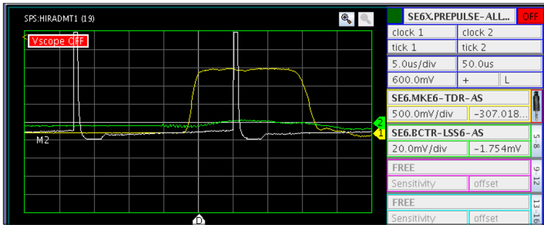
Figure 9.4: Kicker application. White signal shows 12 bunches.
