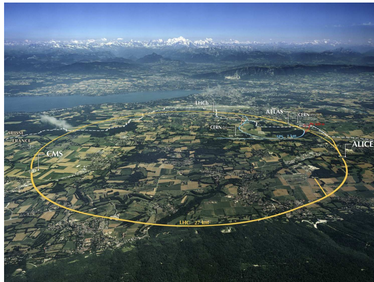
Figure 1.1: CERN aerial view. In yellow, the LHC with its four main experiments. In blue, SPS accelerator. In red, PS accelerator.
