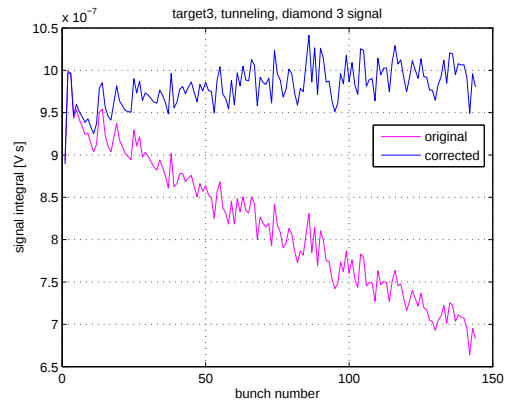
(f) Corrected signal integral for target 3 diamond 3.
