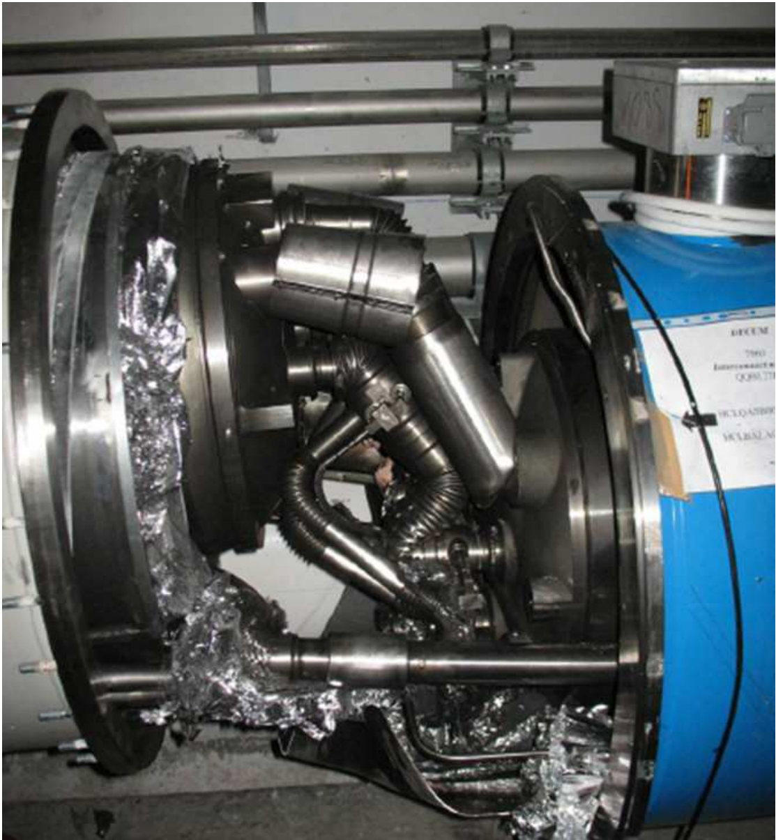
Figure 7.1: Accidental release of the energy stored in the main dipole circuit, 600 MJ in the dipole. (no beam).
