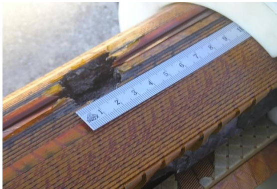
Figure 2.12. Example of damage in the magnet after a not well protected quench
