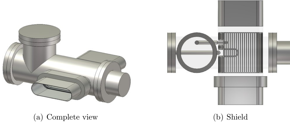
Figure 3.42: The racetrack beam pipe interconnect housing a horizontal and a vertical shielded beam profile scanner for the extracted beam. On the right, the horizontal cut is shown. The beam is passing from bottom to top.
