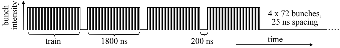
Figure 2.3: The 25 ns SPS beam composition in the time domain.
