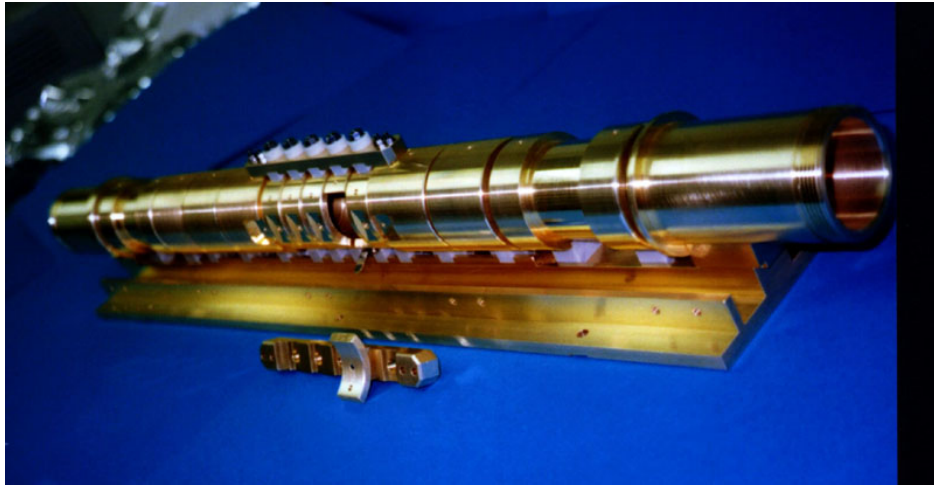
FIGURE 2.16: The MUSASHI multi-ring electrode trap [80].
