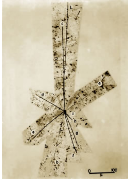
FIGURE 1.2: First observation of an antiproton annihilation event detected using a photographic emulsion at the Bevatron. The antiproton enters from the top of the image (the track labeled as "L") and travels about 430\ \mu\text{m} before the annihilation with a proton producing nine different charged particles 1 .
