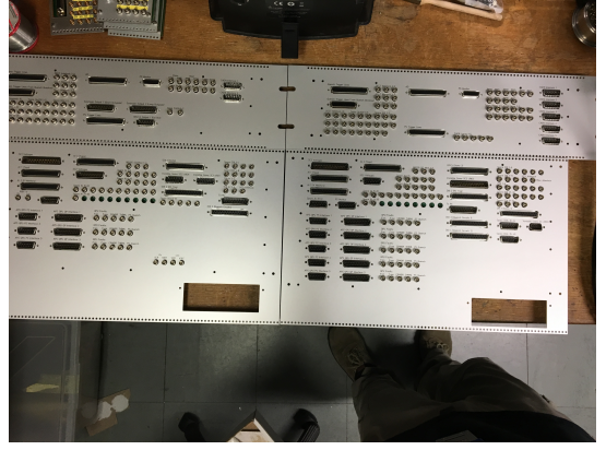
Fig. 3 and 4 Power supply and quench protection breakout circuit boards, with and without front panels.
